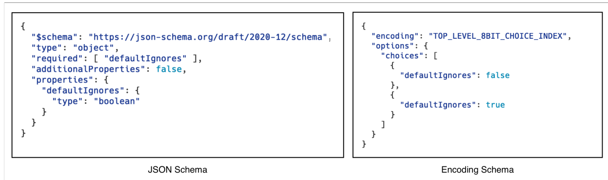
Figure 8.2: An example of an JSON BinPack Encoding Schema. The left side of the figure shows a JSON Schema [159] definition for a JSON [46] object with a single boolean property. The right side of the figure shows the corresponding JSON BinPack Encoding Schema, which flattens the finite possible states of the original schema definition into an 8-bit enumeration that consists of two values. The encoding property refers to an encoding defined by the JSON BinPack Encoder component discussed in subsection 8.3.3 . The TOP_LEVEL_8BIT_CHOICE_INDEX encoding shown in this example and its options are summarized in Table A.2 .
