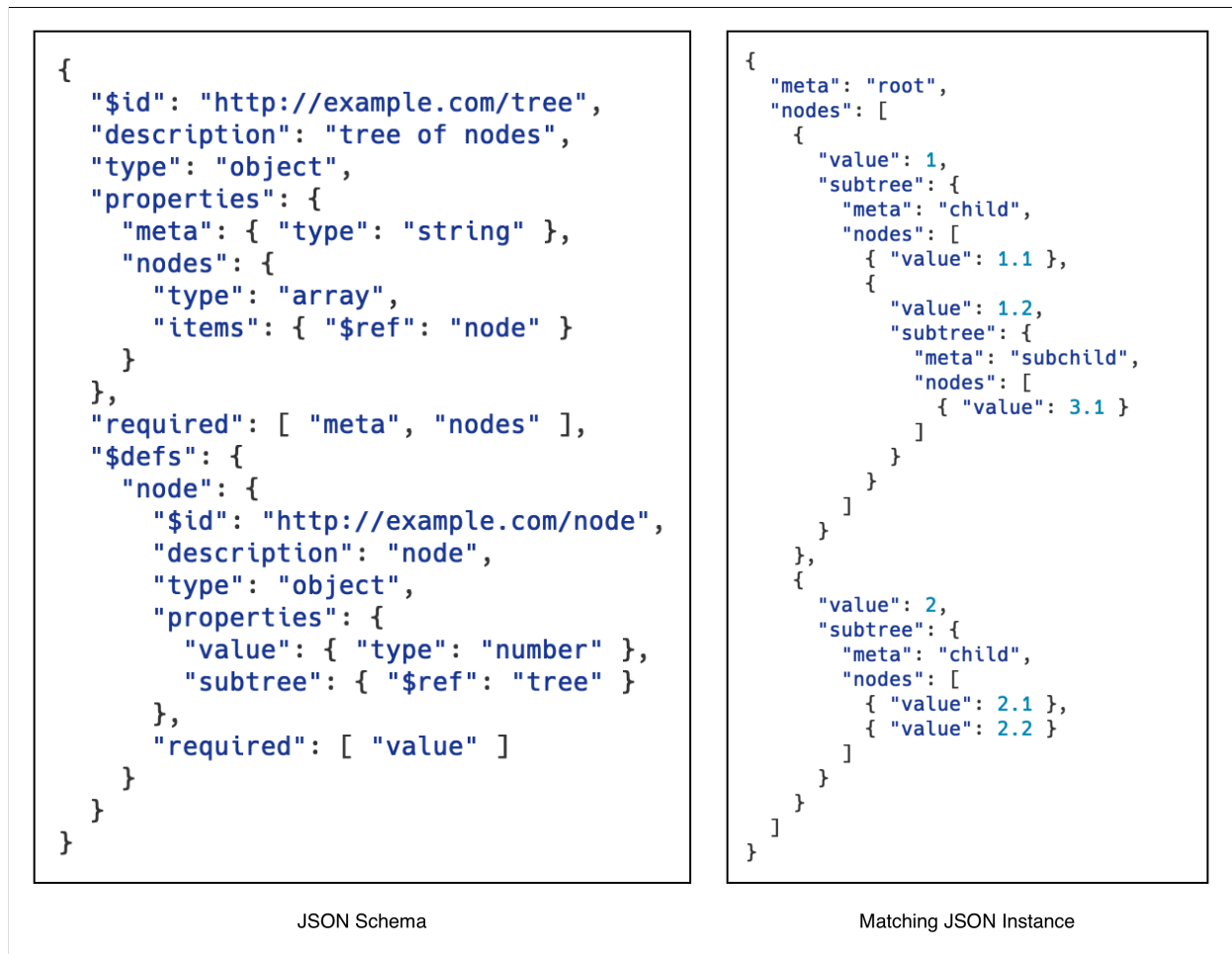
Figure 3.4: On the left, a JSON Schema [159] definition adapted from the official test suite 39 that uses recursive references between schemas to validate arbitrary N-ary tree data structures consisting of real numbers. On the right, an example matching instance.
