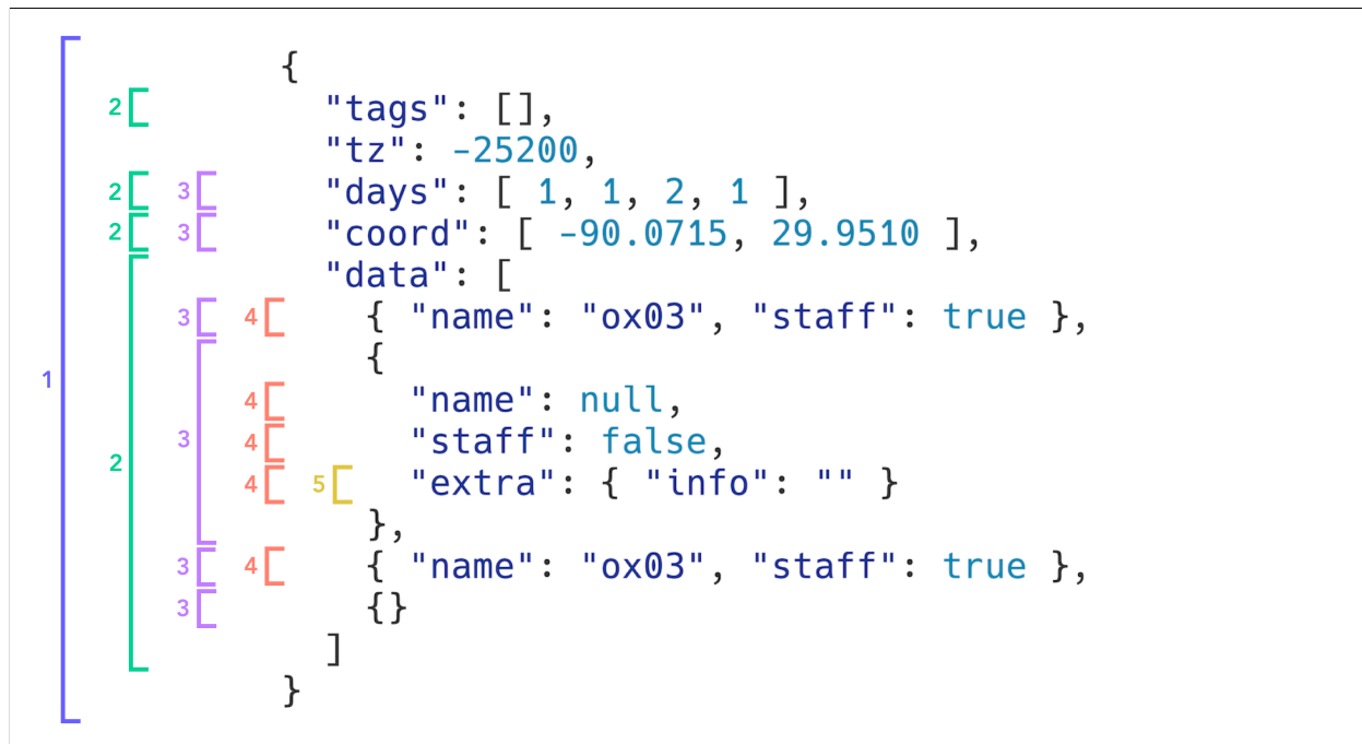
Figure 4.9: An example Tier 2 Minified \geq 100 < 1000 bytes, numeric , non-redundant , and nested JSON document taken from my previous work [151]. The annotations at the left highlight each level in the JSON document. The height of this document is (5 - 1 = 4) (the highest level minus 1).
